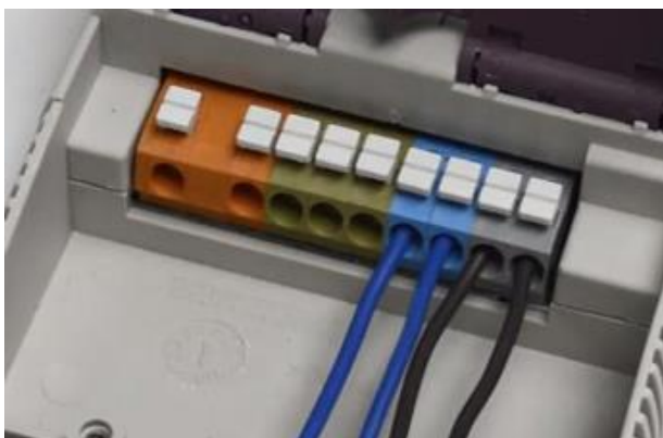
Loop-in loop-out ballast
